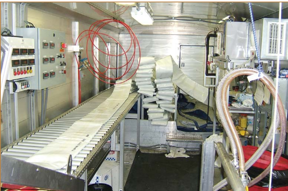
Pro Pipe's specially designed truck is a self-contained CIPP impregnation and installation unit on wheels that enables jobs to be conducted in a timely manner and specific to the most stringent requirements.
